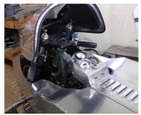
The shape of things to come. This is a partial mock-up of the front fairing incorporating some of the design features currently under consideration. Kind of a mix between a bumper car and a jet fighter! (Hah!)
