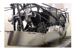
By early December we had completed much of the rear bodywork behind the rider's seat. These slowly receding surfaces will help keep the air flowing around Ted attached and laminar and reduce the size of the turbulent wake at the back of the bike. The area at the rear end of the bodywork (still in cardboard) is only 0.7 square feet.
