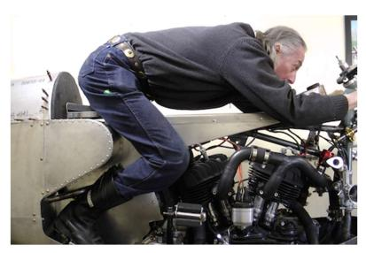
With the gas tank out of the way, Ted's back is now almost perfectly horizontal while he remains on the seat (such as it is). The extra 7" added to the front of the frame (necessary to accommodate the supercharger) provides the added benefit of allowing him to lay down along the top rails without face-planting the steering head. His legs are beneath him in a position of greater control, in the "leg wells" and out of the airstream. He looks a lot like a jockey on a race horse!
