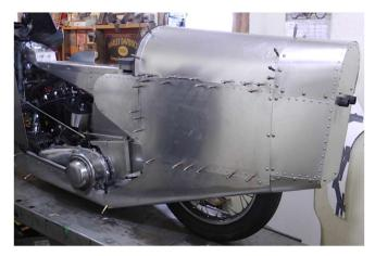
This next photo shows the completion of much of the rear bodywork. Once the front fairing sides are done, Ted's legs will fit into "leg wells" in each side of the bike. This view also shows the new exhaust piping and outlet stubs mentioned in the previous update. The kick starter will be visible outside of the bodywork (with a streamlined "pocket" for the pedal to fit into). It will be a "rocket ship with a kick starter", Hah!
