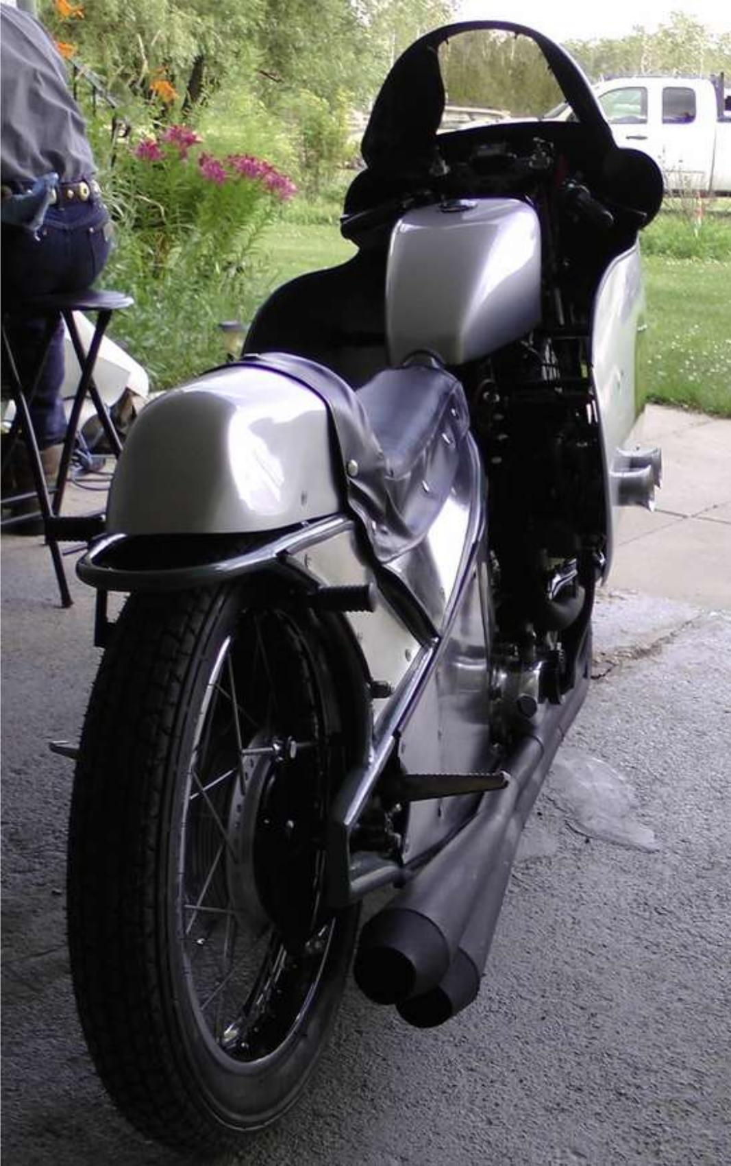
Here's some pics of the racer. The first one highlights the exhaust that Ted fabricated. The header pipes are equal length at 44", which should provide the biggest acoustic hit at ~4600 rpm. Note the contortions that the rear pipe goes through to remain an equal length to the front. Both beautiful and functional... nice job Ted!
