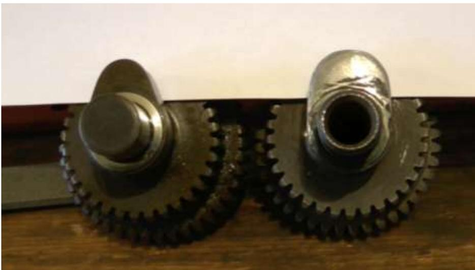
Stock and modified intake cams. Our intakes not only provide much higher lift, but much greater valve openings on both opening and closing ramps.
