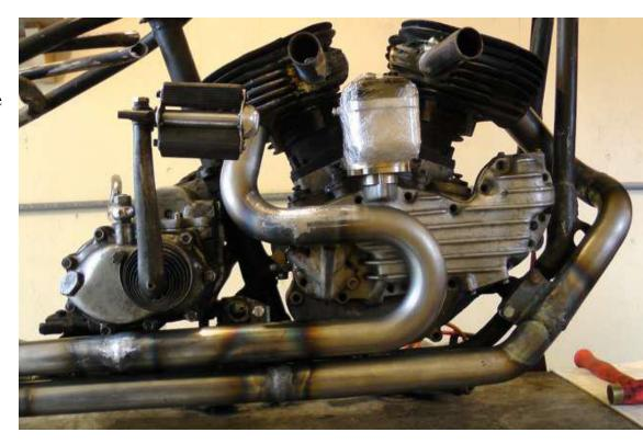
The next pic shows the megaphones. It is estimated that they will spread the acoustic wave effect down ~1000 rpm, so that the engine will start to come on the pipe at about 3600 rpm. However, the greatest wave action will remain at 4600 (reflecting from the entrance to the megaphone / end of the straight pipe). To maximize inertial tuning, the curved part of the headers are 1.625" ID while the
