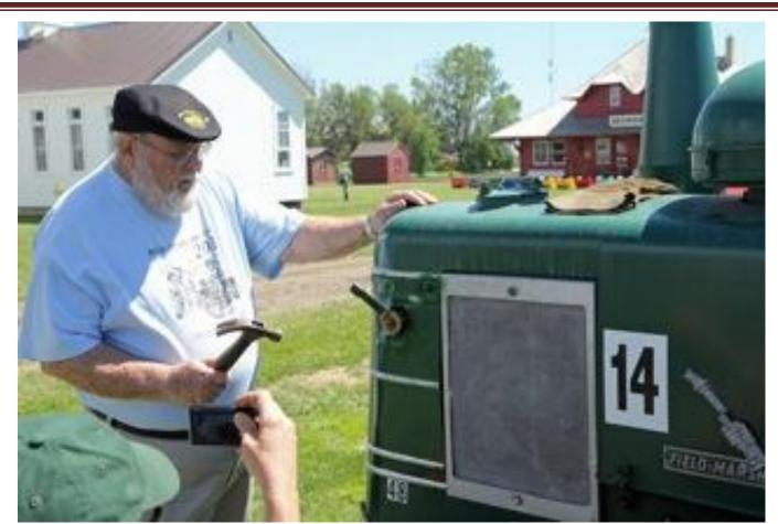
Starting a Tractor with a shotgun shell. Maybe we can use this idea on
